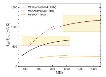
FIG. 2.— The sensitivity of the 'Rebaselined' and 'Alternative' designs for the SKA1-MID receivers, shown as total  $A_{\rm eff}/T_{\rm sys}$  curves for the sub-array. The MeerKAT bands (orange lines) are shown for comparison. The yellow shaded regions denote the SKA1 Baseline specification sensitivity (Dewdney et al. 2013) for the original assumption of 190 dishes (upper limit), and corrected for the post-rebaselining figure of 130 dishes (lower limit).
